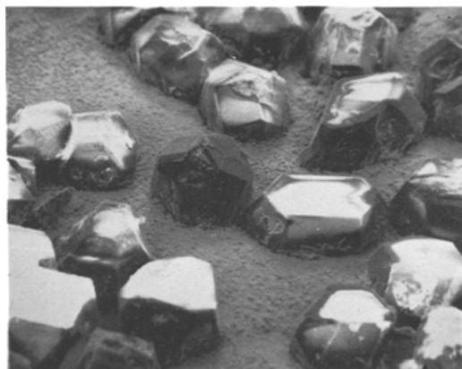
Figure 7 Scanning electron micrograph of the surface of a diamond grit copper-0.73% titanium alloy compact, produced by hot-pressing for 5.0h at 700°C, used to abrade steel sheet for 0.5h, 60°C, \times 120 .
